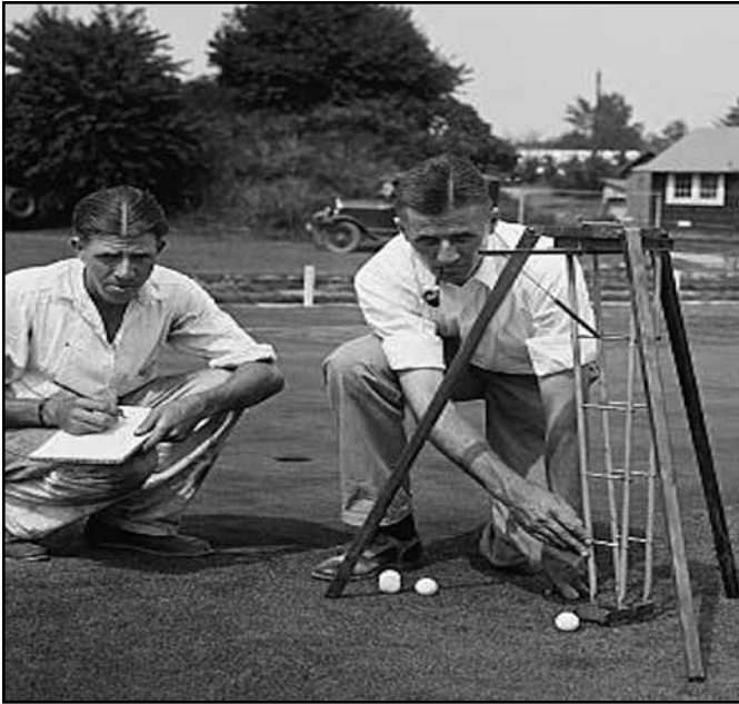
Golf engineers tried many experiments to measure green speed before settling on the simple Stimpmeter, inspired by watching ply at Oakmont.
